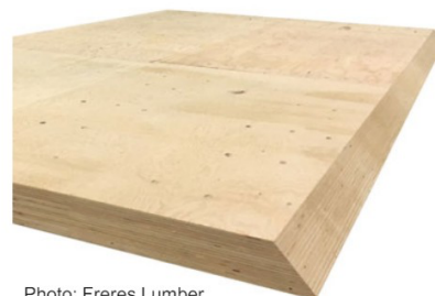
Cross-Laminated Timber (CLT) SCL laminations
